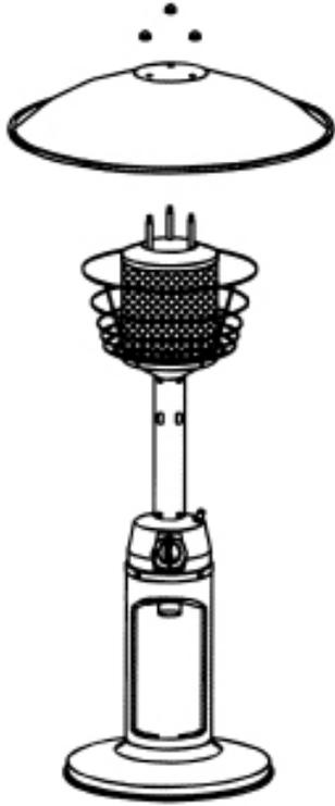
**Step 6 - Rotate regulator toward opening in housing. Line up threads on gas cylinder with those on the regulator. Insert and rotate cylinder clockwise until tight.**
